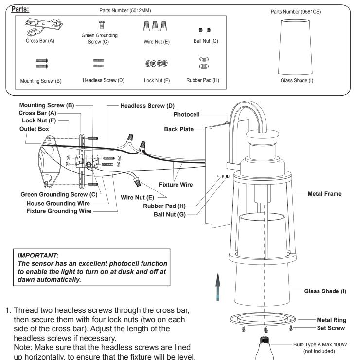
2. Attach the cross bar to the outlet box by using two mounting screws.
