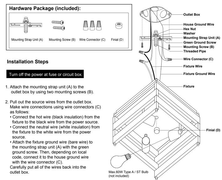
Attach the ceiling pan to the mounting strap unit (A) by inserting threaded pipe into the center hole the ceiling pan and secure it with the finial.
