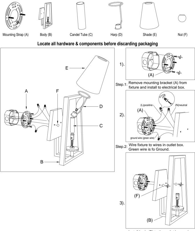
Step.3: Install body (B) to the outlet box and secure with nut(F). Place the Candle Tube (C) over the socket and place Harp (D) on the tube.Install light bulb.Place glass Shade (E) on the harp.
